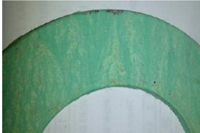
Figure 55: Poor Gasket Conformability
