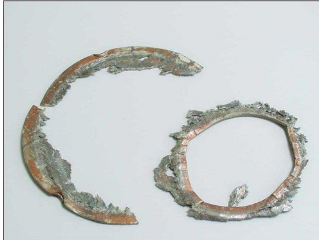
Figure 56: Gasket Chemical Attack
