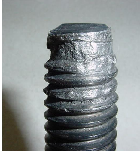
Figure 43: Galled Stainless Steel Bolt
