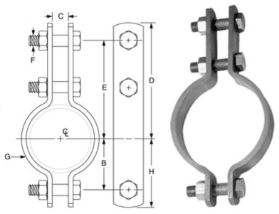
**Note:** This picture is representative of a typical Figure 295. Distance between clamp ears beneath pipe may or may not be equal to upper gap.
